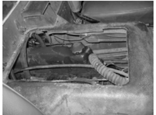
B30 engine visible through access cover between front seats
