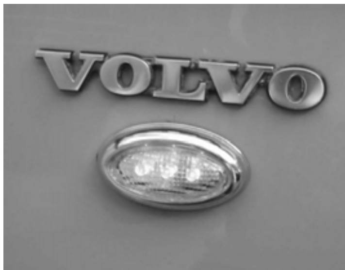
LED Side Repeater light on Thorben's 240. This is the non-genuine one available at Super Cheap
