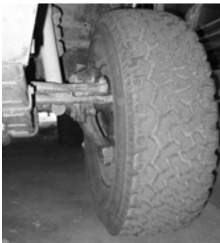
Front axle showing hub gearbox. This is serious off-road machinery
