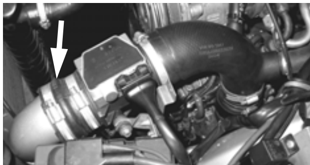
Figure 6: Short Rubber Coupling from Saab 900T
