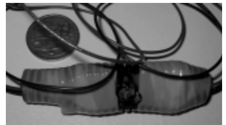
5-volt Power Supply
