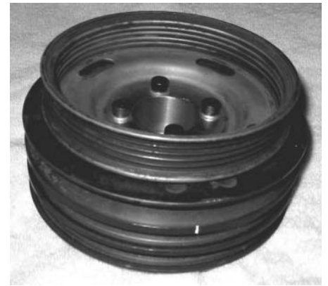
Figure 5: Crank Pulley Assembly
