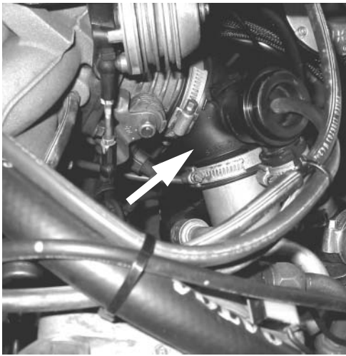
Figure 4: 120-degree Elbow Pipe
