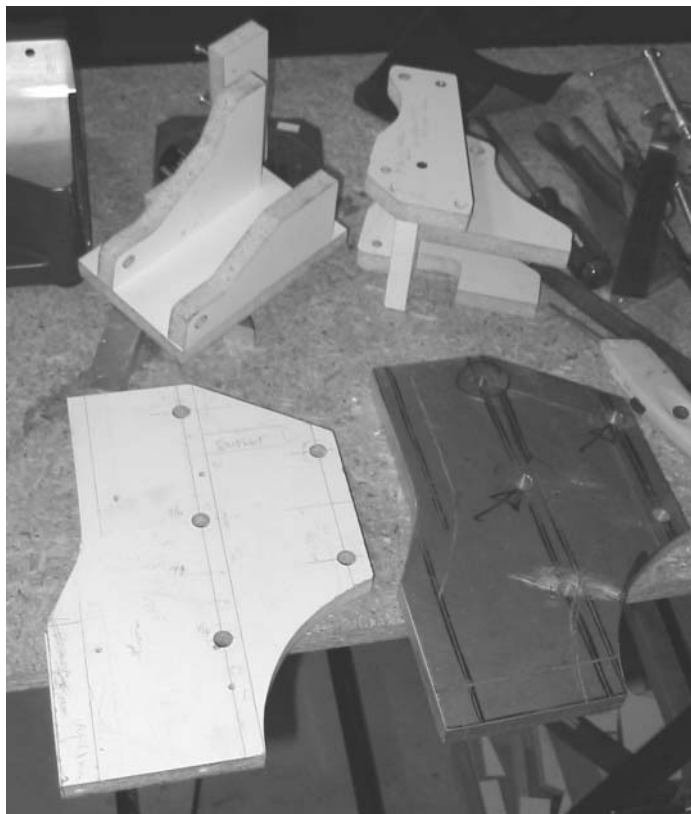
Figure 3: Mk. II Laminate base plate (Left) and Aluminium base plate (Right)
