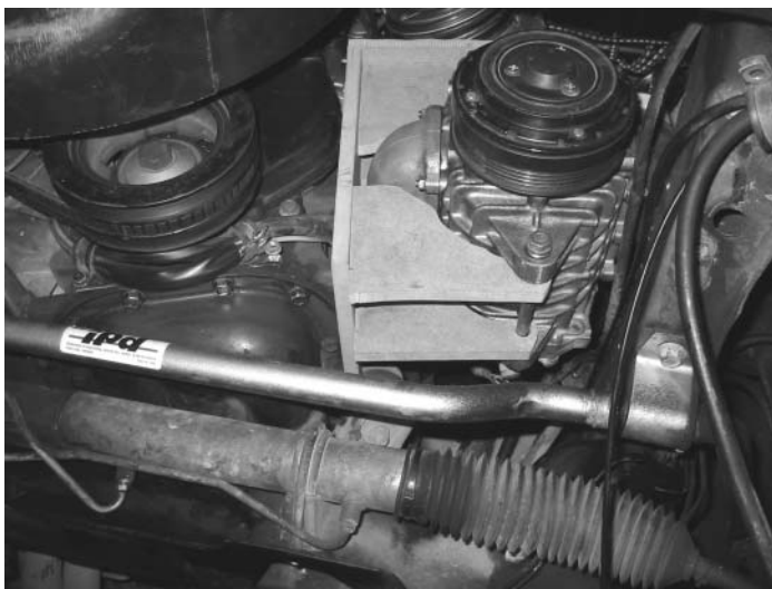
Figure 2: MDF prototype bracket Mk. I bolted on engine
