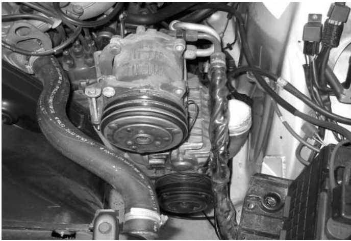
Figure 2: New home for SC below A/C Compressor
